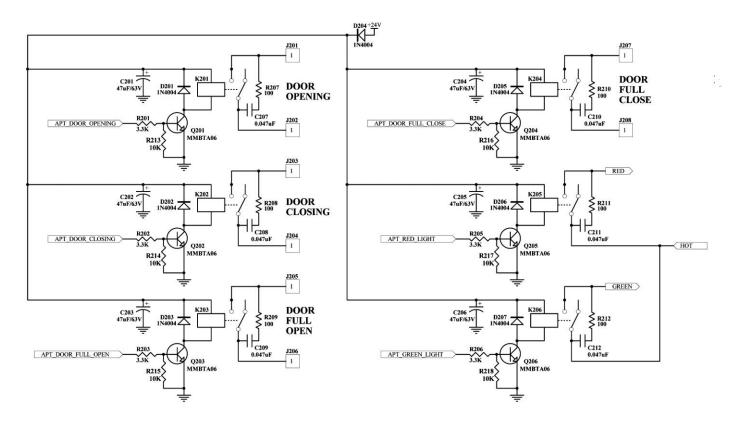
Note: K### in the above design are the relays (there are total of 6 relays in this design).
